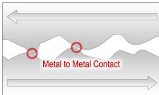
Figure 1: Asperities on touching metal surfaces
