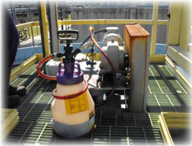
No funnels or opening gear units to add oil
